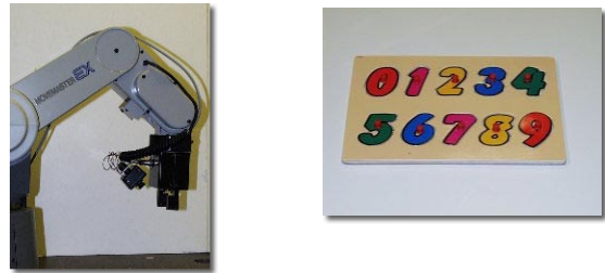
Figure 3. Robot with a hand-mounted camera and a puzzle for pick and place operations.
